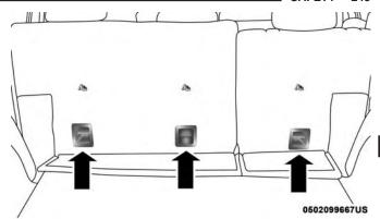
Top Tether Strap Anchorage (Located On Seatback)
