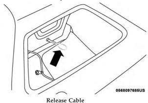
**NOTE:** If the fuel door does not latch after the manual release cable has been activated, the actuator latch should be manually returned to the closed position.
