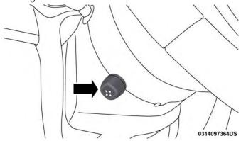
Power Tilt/Telescoping Steering Column
