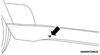
Lift Point Symbol On Sill Molding
