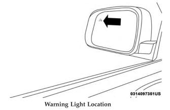
The BSM system monitors the detection zone from three different entry points (side, rear, front) while driving to see if an alert is necessary. The BSM system will issue an alert during these types of zone entries.
