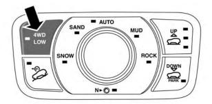
NOTE: If shift conditions/interlocks are not met, or a transfer case motor temperature protection condition exists, a "For 4x4 Low Slow Below 3 mph (5 km/h) Put Trans in "N" Press 4 Low" message will flash from the instrument cluster display. Refer to "Instrument Cluster Display" in "Getting To Know Your Instrument Panel" for further information.
