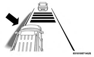
Lane Approached (Flashing Yellow Thick Line, Solid Yellow Thin Line/Flashing Yellow Telltale (2)
