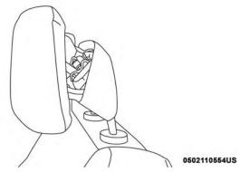
Active Head Restraint (AHR) Deployed
