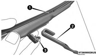
Wiper Blade Removed From Wiper Arm
