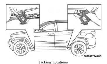
4. For the front axle, place the jack on the body flange just behind the front tire as indicated by the triangular lift point symbol on the sill molding. Do not raise the vehicle until you are sure the jack is fully engaged.
