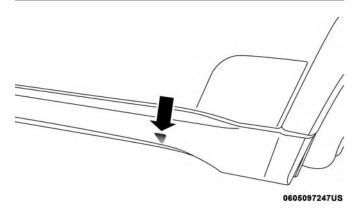
Lift Point Symbol On Sill Molding
