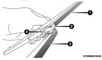
Wiper Blade Removed From Wiper Arm
