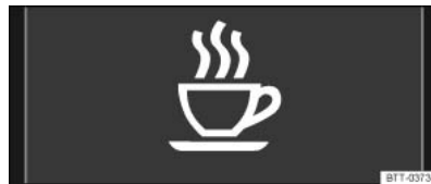
Fig. 18 On the instrument cluster display: Driver Alert System.
