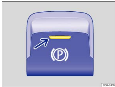
Fig. 151 In centre console: button for the electronic parking brake.
