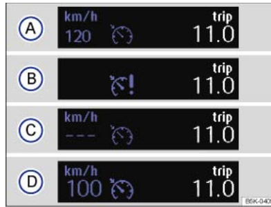
Fig. 136 On the instrument cluster display: cruise control system status displays (illustration).
