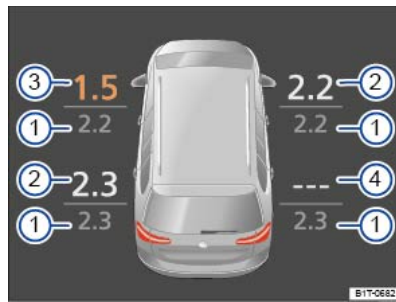
Fig. 234 Typical display in the instrument cluster: current tyre pressures.
