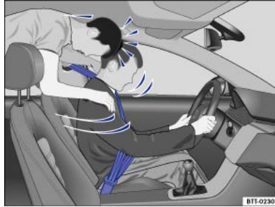
Fig. 36 The unbelted rear passenger is thrown forwards, hitting the belted driver.
