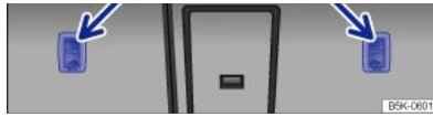
Fig. 57 On the back of the rear bench seat: anchor rings for the top tether.
