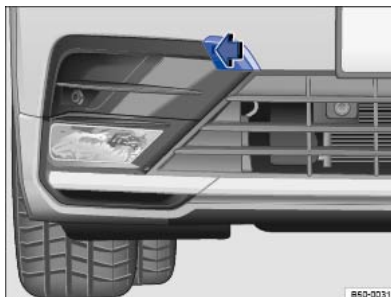
Fig. 221 In the right-hand side of the front bumper: cover for the towing eye mounting.
