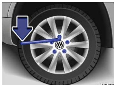
Fig. 244 Changing a wheel: loosening the wheel bolts.
