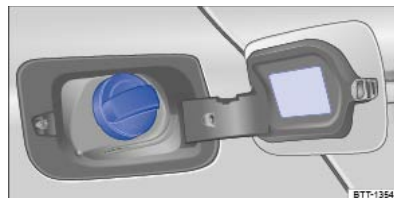
Fig. 195 Behind the tank flap: tank cap.
