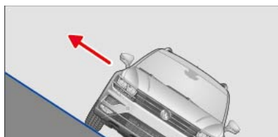
Fig. 133 Steering downhill along the maximum gradient.
