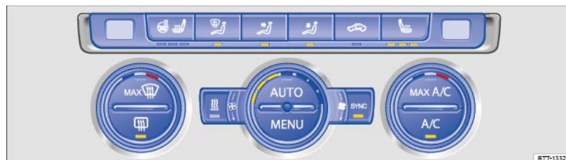
Fig. 109 In the upper section of the centre console: controls for the manual air conditioning system.
