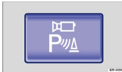
Fig. 160 In the centre console: button for manually switching on Area View.
