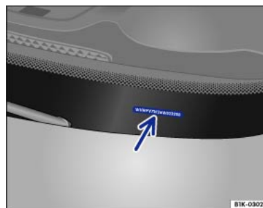
Fig. 254 In the windscreen: vehicle identification number.
