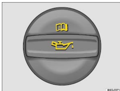
Fig. 228 In the engine compartment: engine oil filler cap (illustration).
