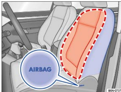
Fig. 48 On the side of the front seat: location and deployment zone of the side airbag.
