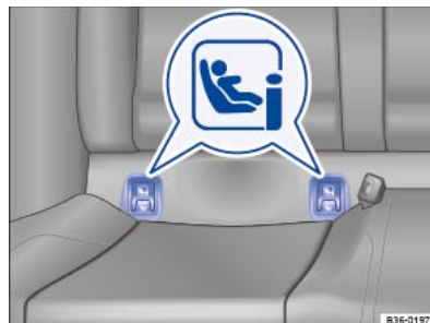
Fig. 55 On vehicle seat: markings identifying the ISOFIX anchoring points for child seats.
