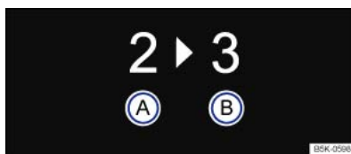
Fig. 115 On the instrument cluster display: gear-change indicator.
