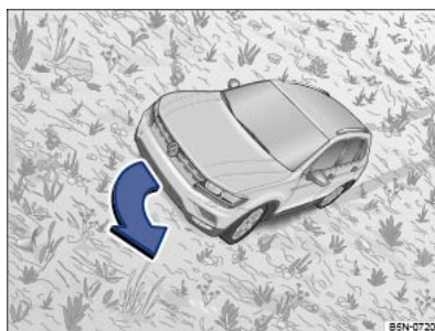
Fig. 133 Steering downhill along the maximum gradient.
