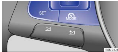
Fig. 137 Left-hand side of the multifunction steering wheel: buttons for operating the cruise control system.
