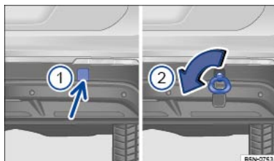
Fig. 219 On the right-hand side of the rear bumper: screwed-in towing eye.
