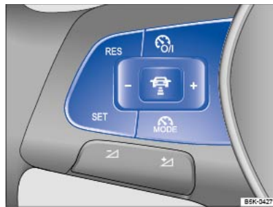
Fig. 145 Left-hand side of the multifunction steering wheel: buttons for operating ACC
