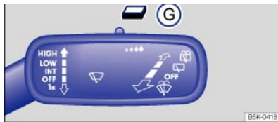
Fig. 102 On the left of the steering column: operating the rear window wiper.
