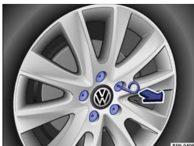
Fig. 243 Removing the wheel bolt caps.
