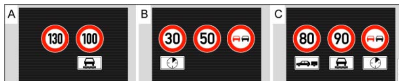
Fig. 19 On the instrument cluster display: examples of recognised speed limits or overtaking restrictions with accompanying additional signs.
