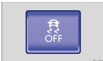
Fig. 162 In the centre console: button for switching TCS on and off manually.
