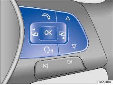
Fig. 25 Right-hand side of the multifunction steering wheel: controls for using the menus and information displays in the instrument cluster.
