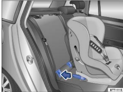
Fig. 56 Fitting a typical ISOFIX child seat with the attachment arms.
