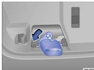
Fig. 75 In the luggage compartment: manual release for the boot lid.
