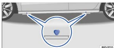
Fig. 246 Lifting points for the jack.
