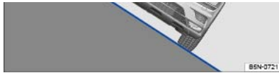
Fig. 134 On steep slopes, you should always use the doors pointing up the hill to get out of the vehicle.
