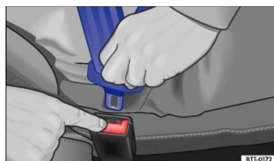
Fig. 38 Inserting the seat belt latch plate into the buckle.
