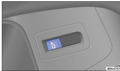
Fig. 71 In the driver door: release button for the boot lid.
