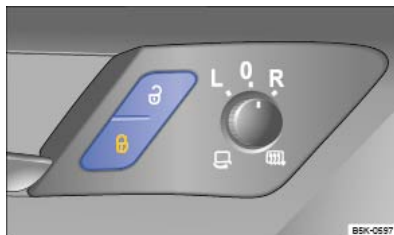
Fig. 64 In the driver door: central locking button.
