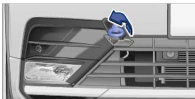
Fig. 221 In the right-hand side of the front bumper: cover for the towing eye mounting.
