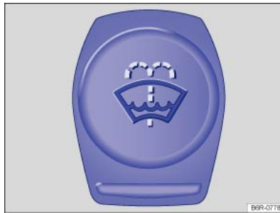
Fig. 226 In the engine compartment: cap of washer fluid reservoir.
