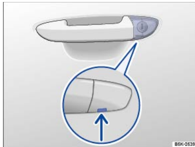
Fig. 69 Driver door handle: concealed lock cylinder
