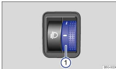
Fig. 100 Next to steering wheel: headlight range control ①.
