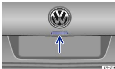
Fig. 72 In the boot lid: button for opening the boot lid.
