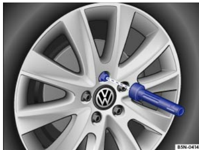
Fig. 248 Changing the wheel: removing the wheel bolts with the screwdriver handle.
