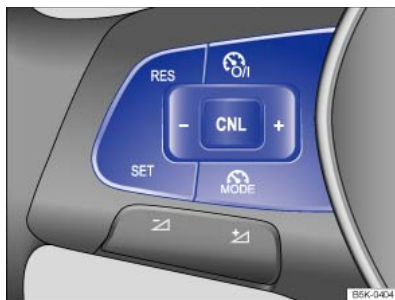
Fig. 141 Left-hand side of the multifunction steering wheel: buttons for operating the speed limiter.
