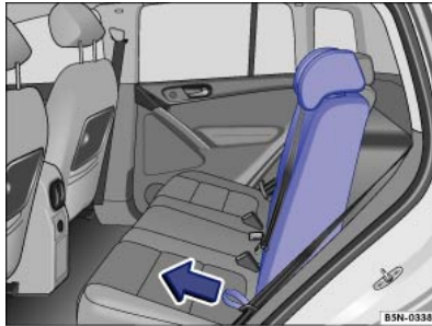
Fig. 86 Folding the backrest forwards and backwards.
