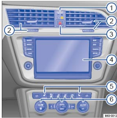
Fig. 10 Overview of the upper section of the centre console.
