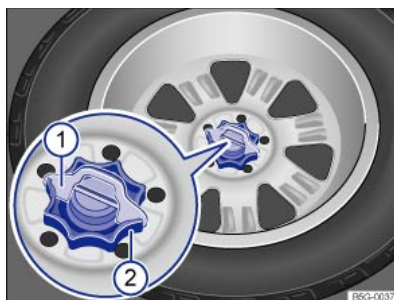
Fig. 239 In the luggage compartment: handwheel for securing the spare wheel.
