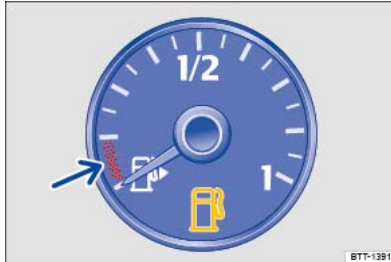
Fig. 20 In the instrument cluster: fuel gauge for petrol and diesel.
