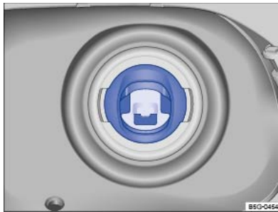
Fig. 196 In the tank filler neck: misfuelling prevention device.
