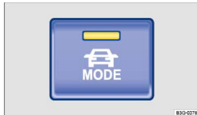
Fig. 128 In the lower section of the centre console: driving profile selection button.
