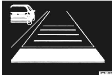
Fig. 142 On the instrument cluster display: slower vehicle detected in the left-hand lane (illustration).
