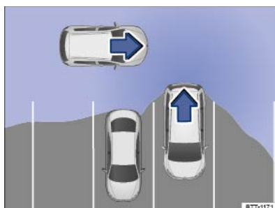
Fig. 149 Rear Traffic Alert: monitored area around the vehicle leaving the parking space.
