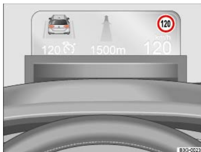
Fig. 17 On the dash panel above the steering wheel: examples of information shown in the Head-up Display.
