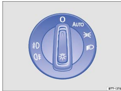
Fig. 97 Next to the steering wheel: light switch (one variant).
