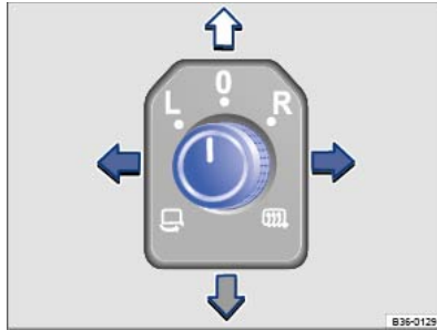
Fig. 106 In the driver door: rotary knob for the exterior mirrors.
