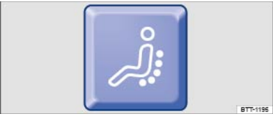
Fig. 95 In the lower area of the driver seat: button for massage function.
