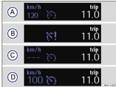
Fig. 138 On the instrument cluster display: cruise control system status displays (illustration).
