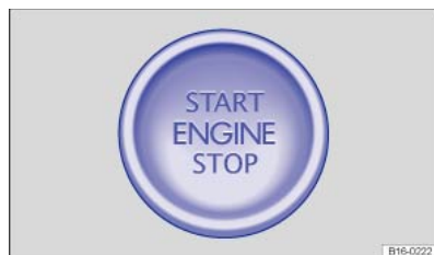
Fig. 119 In the lower section of the centre console: starter button for starting the engine.
