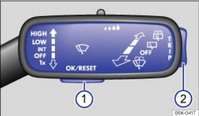
Fig. 24 On the right of the steering column: buttons on the wiper lever (illustration).
