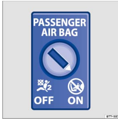
Fig. 46 In the dash panel on the front passenger side or in the stowage compartment: key-operated switch for switching the front passenger front airbag on and off.
