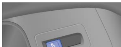
Fig. 64 In the driver door: central locking button.
