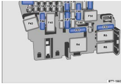
Fig. 211 In the dash panel: fuse layout.
