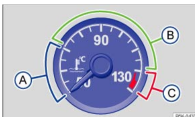
Fig. 21 In the instrument cluster: coolant temperature display (illustration).
