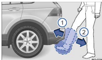
Fig. 73 Sensor-controlled luggage compartment opener (Easy Open).
