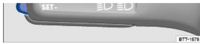
Fig. 139 On the left of the steering column: switch and buttons for operating the speed limiter.
