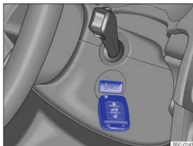
Fig. 120 On the right of the steering column: emergency start function in vehicles with the Keyless Access locking and starting system.
