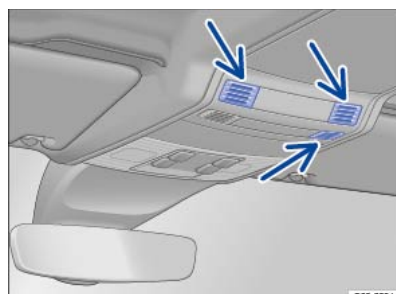
Fig. 67 In the roof console: sensors for the interior monitoring system (arrows).
