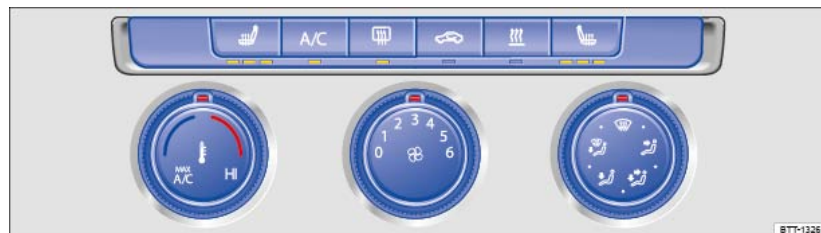
Fig. 109 In the upper section of the centre console: controls for the manual air conditioning system.
