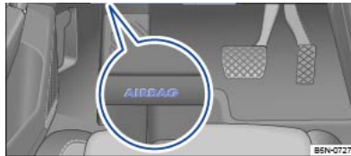
Fig. 50 On the driver side: location of the knee airbag
