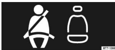
Fig. 32 On the instrument cluster display: seat belt status for the rear seats.
