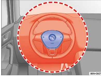
Fig. 44 Location and deployment zone of the driver front airbag.
