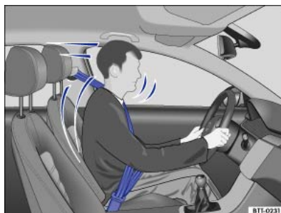
Fig. 37 Driver restrained by a properly positioned seat belt during a sudden braking manoeuvre.
